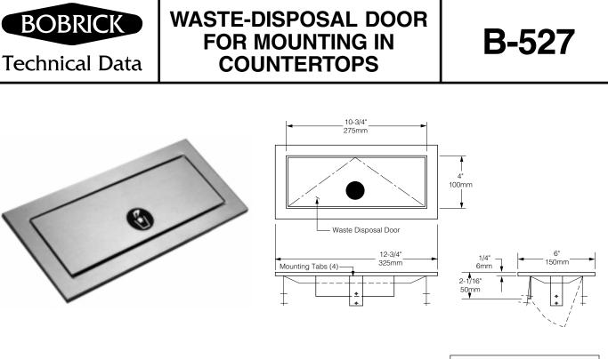
Rough Countertop Cutout 11-1/4" (285mm) wide 4-1/2" (115mm) high 3/4" to 1-1/2" (19 to 38mm) mounting thickness 4-1/2" (115mm) minimum clearance below mounting surface
